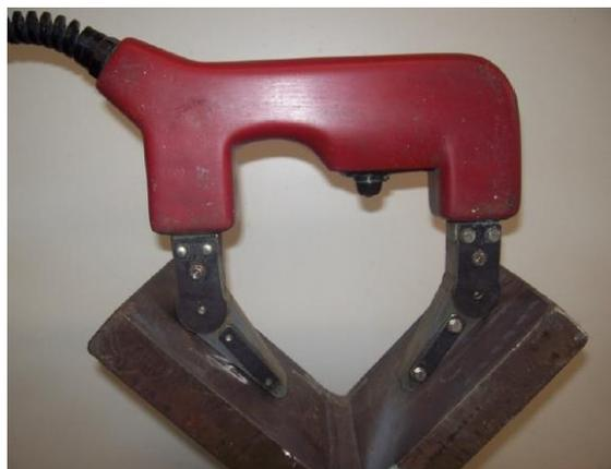
Figure 4 - Magnetization with the manual yoke magnet
