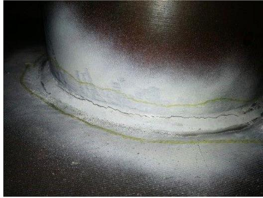
Figure 8 -Representation of the steps performed on the liquid penetrant testing
