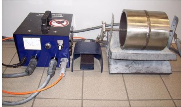
Figure 5 - Magnetization via current-carrying conductors
