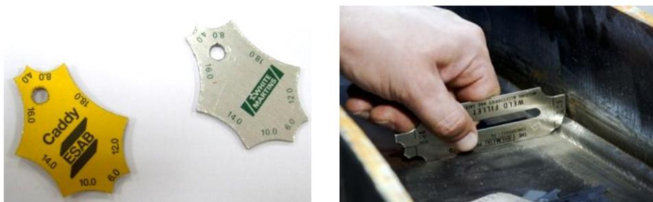
Figure 9 - Gauge for checking fillet weld profile
