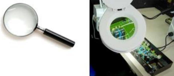
Figure 2 - Manual and fixed magnifier
