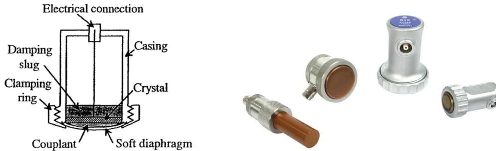
Figure 9 - Straight Beam Contact Transducer
