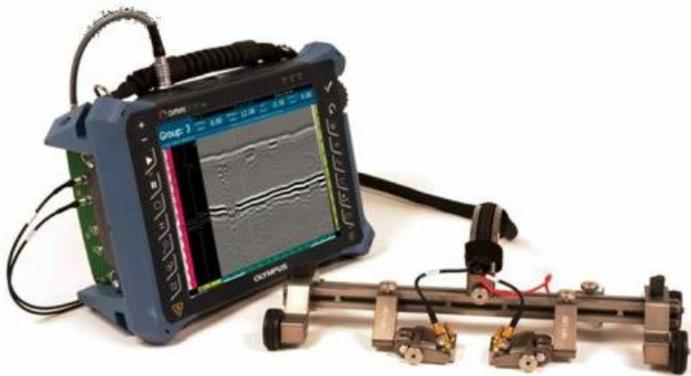
TOFD Caliper - Compact Single Axis Scanner
