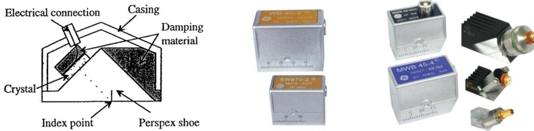
Figure 11 - Angle Beam Contact Transducers
