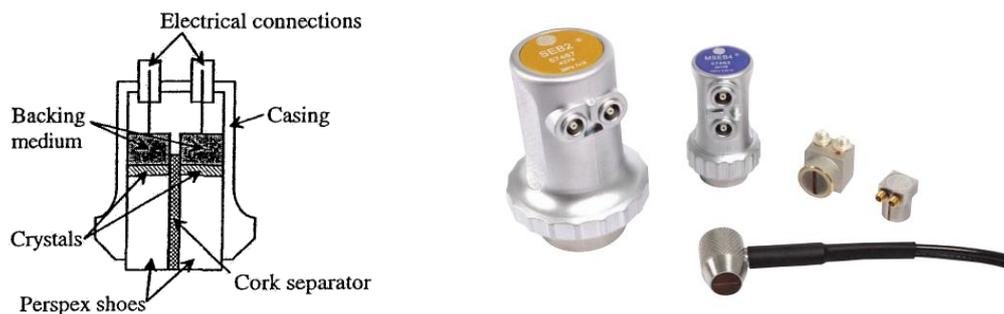
Figure 10 - Transducers, Straight-Beam Dual Element TR
