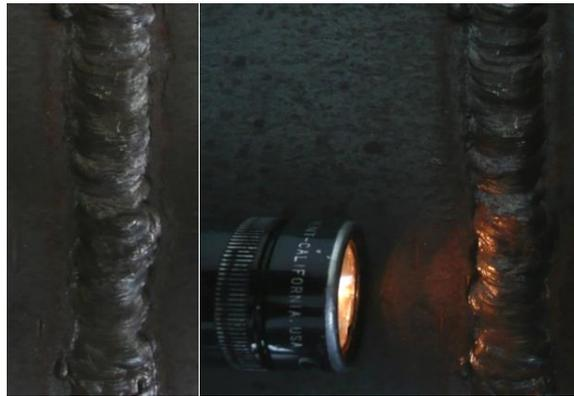
Figure 3 - Localisation of undercut by projecting its shadow
