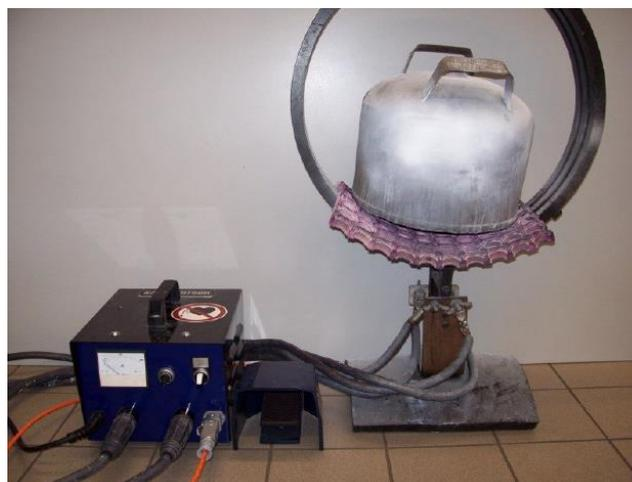
Figure 7 - Magnetization via coils
