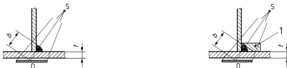
a) Arrangement for testing without compensating edge
