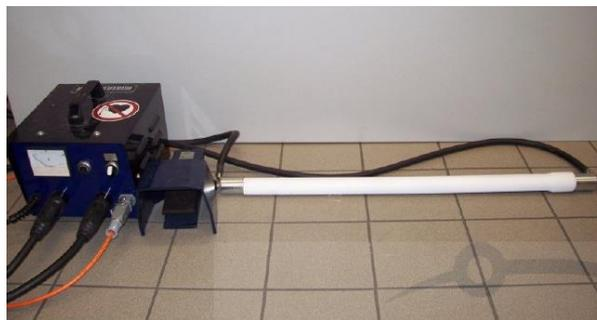
Figure 6 - Magnetization via current flow
